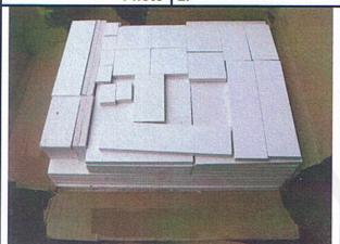
"BESTA" Magnesium Oxide (MgO) boards of thickness 16mm, cut to the required size were received on 03/11/2008.
