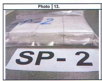
Physical and Mechanical Properties – Linear Thermal shrinkage test .
