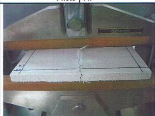
Physical and Mechanical Properties – Bending Strength test.
